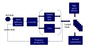
Fig 3.1 Block diagram of Hybrid DLL Model
