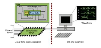
Fig 1. Trace-based debugging
