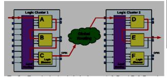
Fig 7 Example signal path; logic elements A & B and D & F can be incrementally swapped for greater trace-flexibility.
