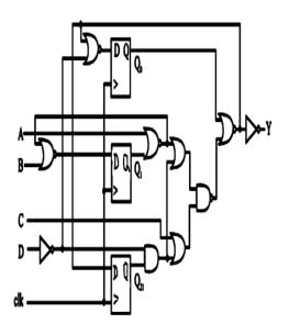
Fig 3. Circuit Diagram for Trace buffer
