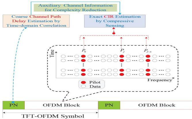
Figure 1: Proposed frame structure and the corresponding CS-based CE for the TFT-OFDM scheme.
