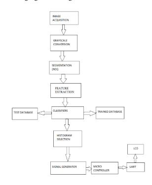
A histogram is a graphical representation of the distribution of data. The signal generator is used to generate a signal according to the histogram results. The generated signal is sent into microcontroller AT89S52 which is connected with UART and the output signal is fed into LCD to display whether the person is authenticated or not.
